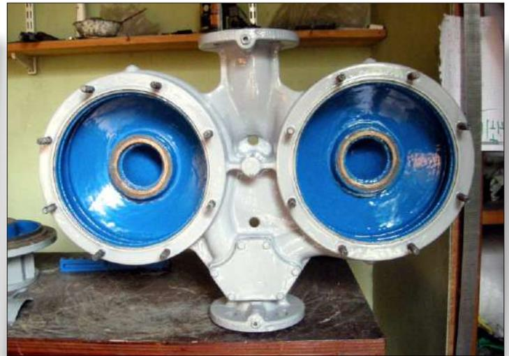
After thoroughly grit blasting, all deeply damaged areas were repaired with CeramAlloy CP+AC. Two coats of CeramAlloy CL+AC were then applied to provide erosion / corrosion resistance.
